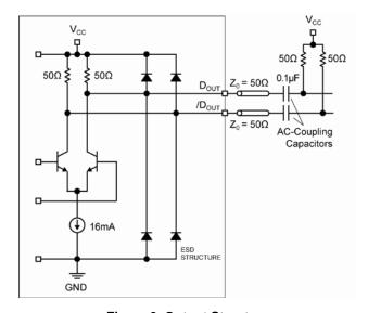
Figure 3. Output Structure
