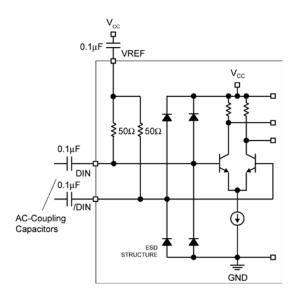
Figure 2. Input Structure
