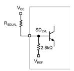
Figure 6.  $SD_{LVL}$  Setting Circuit
