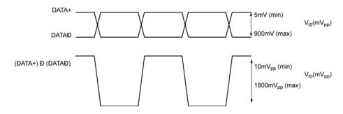
Figure 1.  $V_{IS}$  and  $V_{ID}$  Definition
