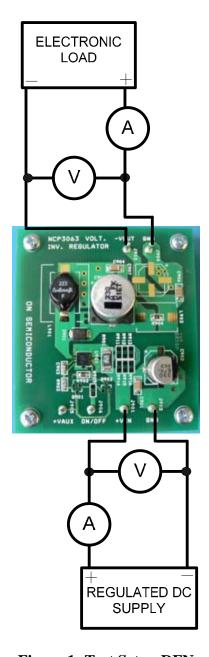
**Figure 1: Test Setup DFN**
