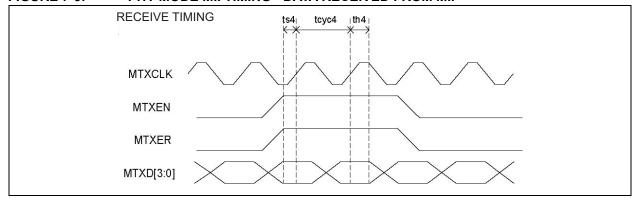
FIGURE 7-6: PHY MODE MII TIMING - DATA TRANSMITTED FROM MII
