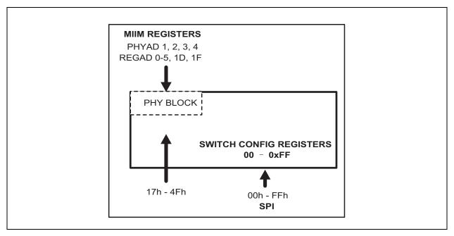
The registers within the linear 0x00-0xFF address space are all accessible via the SPI interface by a CPU attached to that bus. The mapping of the various functions within that linear address space is summarized in Table 4-1.
