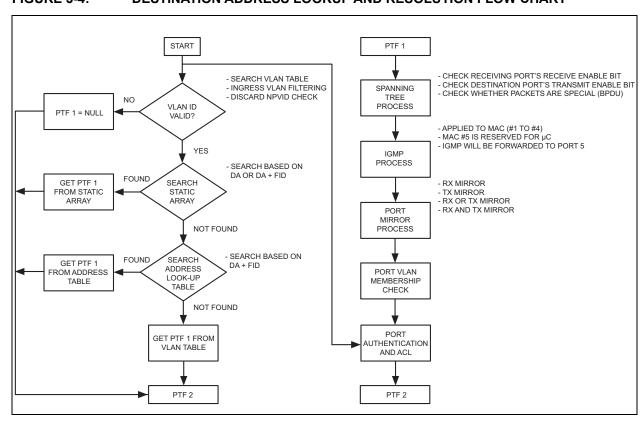
FIGURE 3-4: DESTINATION ADDRESS LOOKUP AND RESOLUTION FLOW CHART
