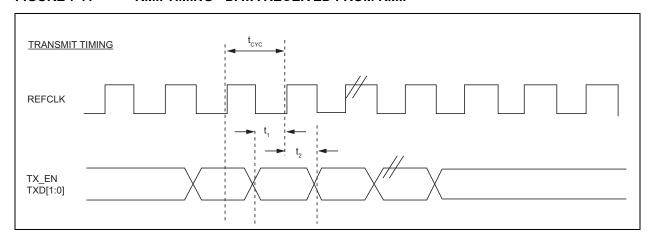
FIGURE 7-8: RMII TIMING - DATA TRANSMITTED FROM RMII
