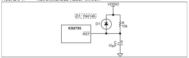
FIGURE 8-2: RECOMMENDED CIRCUIT FOR INTERFACING WITH CPU/FPGA RESET
