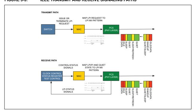
FIGURE 3-5: IEEE TRANSMIT AND RECEIVE SIGNALING PATHS
