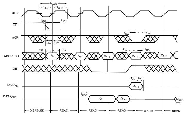
47.  $\overline{CE}_0 = \overline{B0} - \overline{B3} = R/\overline{W} = LOW$ ;  $\overline{CE}_1 = \overline{CNTRST} = \overline{MRST} = CNT/\overline{MSK} = HIGH.$  When  $R/\overline{W}$  first switches low, since  $\overline{OE} = LOW$ , the Write operation cannot be completed (labelled as no operation). One clock cycle is required to three-state the I/O for the Write operation on the next rising edge of CLK.
