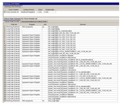
Note that the beginning of the critical chain, on line 1, has Retiming Restriction listed in the **Path Info** column. Also, the end of the critical chain, on line 37, has Retiming Restriction listed also. The retiming restrictions are because of the asynchronous resets on the two registers.
