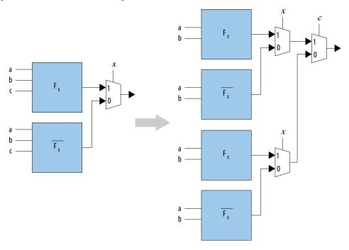
Shannon's decomposition can be an effective optimization technique for loops. When you perform Shannon's decomposition on logic in a loop, the logic in the loop moves outside the loop. The Hyper-Retimer can now pipeline the logic moved outside the loop.
