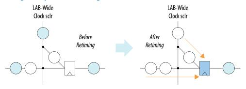
Because the register on the synchronous clear path is shared with other registers, the register splits on the path to other synchronous clear ports as well.
