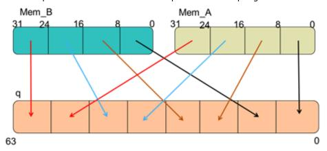
The following RTL examples implement the extra stage to descramble the data from memory on the read side.
