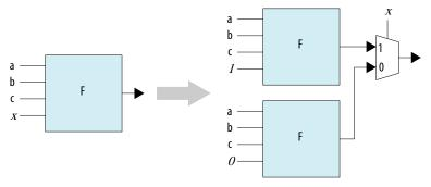
Logic synthesis can take advantage of the constant-driven inputs and slightly reduce the cofactors, as shown in the following diagram.
