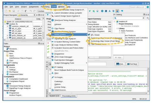
You can also right-click a critical chain in the **Retiming Limit Details** panel in the Hyper-Retimer report, and choose **Locate Critical Chain**. The following images compare the netlist views before synthesis (RTL Viewer), after the Fitter but before the Hyper-Retimer (Technology Map (Post-Fit) Viewer), and after the Hyper-Retimer (**Post-Hyper-Retimer Viewer Showing Bypassed Flipflops**).
