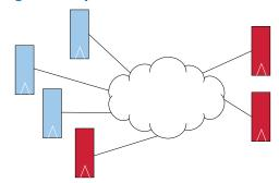
In this case, you can add latency at the boundary of the red clock domain as shown in the figure below, as long as you do not add registers on a red to red domain path. Otherwise, the paths become unbalanced, potentially breaking the design functionality. Although technically possible, it is risky to add latency in this scenario. Before doing so, thoroughly analyze the various paths.
