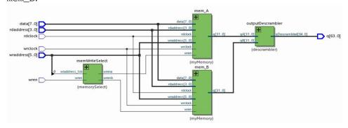
Because of the scheme that controls writing to the memories, you must take care in reconstructing the full 64-bit output during a write. You must account for the interleaving of the individual 8-bit words in the two memories.
