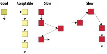
Be realistic about timing margin when building your design. An Intel FPGA comprises a common pool of physical resources. Portions of the design make contact and distort one other as logic is added to the system. Adding stress to the system is typically detrimental to speed. As a design project progresses, there are more ways to slow the system down than to speed it up. Allowing more timing margin at the start helps mitigate this problem.
