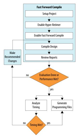
Depending on your work flow, you can run Fast Forward Compile automatically during every compilation, or you can run Fast Forward Compile as a separate process. For example, automating Fast Forward Compilation helps when iterating through various RTL changes. Conversely, when not focusing on design performance, such as when performing board layout or pin and interface planning, save time by disabling Fast Forward Compile.
