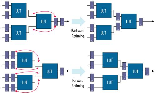
When the Hyper-Retimer cannot retime a register, this is known as a retiming restriction. Such restrictions limit the design's  $f_{MAX}$ . Minimize retiming restrictions in performance-critical parts of your designs to achieve the highest performance.
