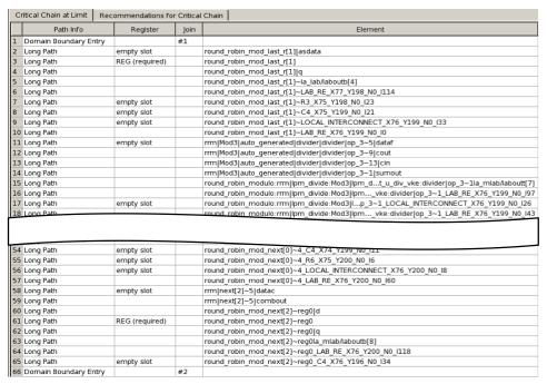
The 66 elements in the critical chain above, correspond to the circuit diagram below with 13 levels of logic. The modulus operator contributes significantly to the low performance. Nine of the 13 levels of logic are part of the implementation for the modulus operator.
