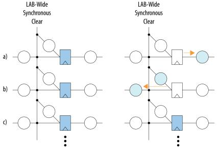
During retiming, the top register in row (a) is pushed right into a Hyper-Register. This is achieved by bypassing the ALM register, but still using the SCLR logic that feeds that register. When the LAB-wide SCLR signal is used, an ALM register must exist on the data path, but it does not have to be used.
