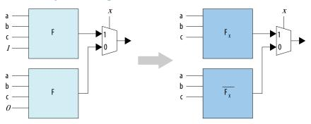
In Hyper-Optimization, the advantage of Shannon's decomposition is that it pushes the x signal to the head of the cone of input logic, making the x signal the fastest path through the cone of logic. The x signal becomes the fastest path at the expense of all other signals. Using Shannon's decomposition also doubles the area cost of the original function.
