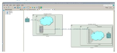
The example design has four banks of registers, a wide AND gate, and two output register stages.
