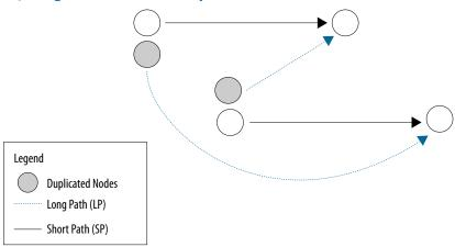
The fitter and Hyper-Retimer can optimize the newly-independent segments separately. The duplicated registers have common sources themselves, so they are not completely independent, but the optimization is easier with an extra, independent register in each part of the critical chain.
