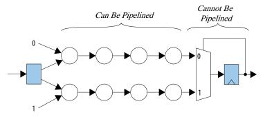
Performing Shannon's decomposition on the logic in the loop reduces the amount of logic in the loop. The Hyper-Retimer can now perform Hyper-Retiming or Hyper-Pipelining on the logic removed from the loop, and increase the circuit performance.
