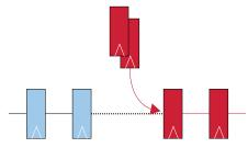
The following figure shows a domain crossing structure that is not recommended for use in Stratix 10 designs, but may exist in designs that target other device families:
