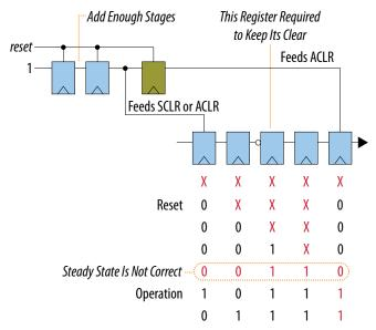
To avoid non-naturally resetting logic because of inverting functions, validate the output to synchronize with reset removal. Then, as long as the validating pipeline can enable the output when the computational pipeline is actually valid, the behavior is equivalent with reset removal. This process is suitable even if the computation portion of the circuit does not naturally reset.
