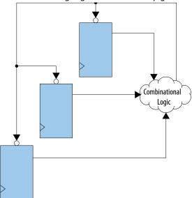
Use loops to save area through hardware re-use. Components that are re-used over several cycles typically involve loops. For example reused components include CRC calculations, filters, floating point dividers, and word aligners. Loops are also used in closed loop feedback designs such as IIR filters and automatic gain control for transmitter power in remote radiohead designs.
