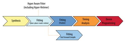
After the Hyper-Retimer or Fast Forward Compile steps, view the results in the Compilation Report to evaluate performance and determine where to implement key RTL performance improvements. After implementing any RTL changes, recompile the design and rerun Fast Forward Compile until performance and timing analysis results are satisfactory.
