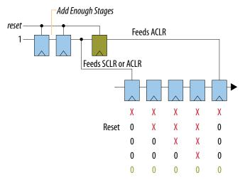
Cases involving inverting logic generally require additional synchronous clears to remain in the pipeline.
