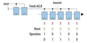
After removing the reset and applying the clock, the register outputs do not settle to the reset state, as in the circuit above. Rather, the inverting register cannot have its asynchronous clear removed to be equivalent to the above circuit after settling out of reset.
