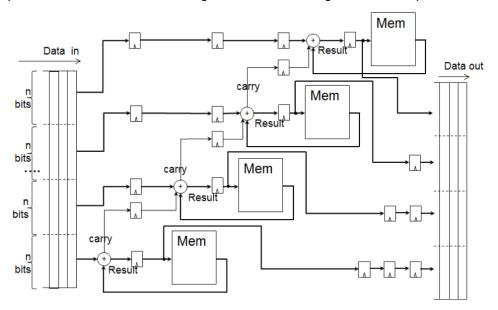
Data words are split into multiple n-bit chunks, where each chunk is small enough to be processed efficiently in one clock cycle. For the best performance, each chunk must be no wider than one M20K memory block.
