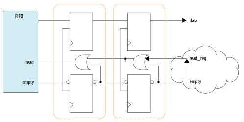
If you have loops involving FIFO control signals, and they are broadcast to many destinations for flow control, you should carefully consider whether there is a way to eliminate the broadcast signals. Pipeline broadcast control signals, and use almost full and almost empty status bits from FIFOs.
