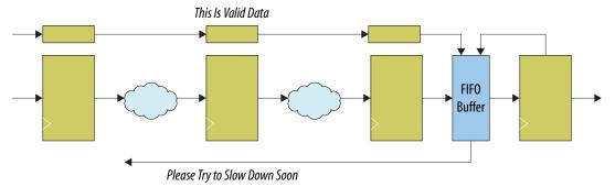
The goal is for data to reach the FIFO buffer every clock cycle. An extra bit of information decides whether the data is valid and should be stored in the FIFO buffer. The critical signal now resides between the FIFO buffer and the downstream register that consumes the data. This loop is much smaller. You can now use pipelining and register retiming to optimize the section upstream of the FIFO buffer.
