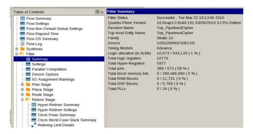
Of the 10770 logic registers after the placement and routing completes, 9089 remain in ALMs. This data means that 1681 (1077 - 9089) registers retime into Hyper-Registers in the HyperFlex fabric. During retiming, a total of 5977 Hyper-Registers implement the 1681 that retime out of ALMs. Again, these values are informational only and does not affect changes you make to your RTL or settings.
