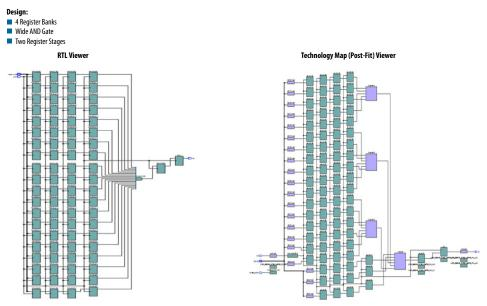
After retiming, the second stage of the register banks is retimed forward into the first bank of Hyper-Registers. The third and fourth stages are retimed forward across AND gates (shown in purple) into Hyper-Registers. The first output stage is moved to a Hyper-Register (the right-most register shown in pink).
