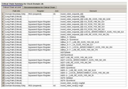
Both the input and output registers are indicated as Domain Boundary Entry because the Fast Forward Compile could insert register stages at these boundaries if Hyper-Pipelining were enabled. Because the critical chain for the base compile does not contain any Fast Forward optimizations, no additional register stages were inserted at either the input to the chain, or the output of the chain.
