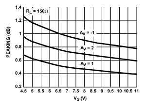
FIGURE 12. PEAKING vs SUPPLY VOLTAGE
