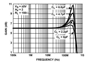
FIGURE 5. FREQUENCY RESPONSE FOR VARIOUS  $C_L$
