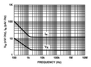
FIGURE 9. VOLTAGE AND CURRENT NOISE vs FREQUENCY
