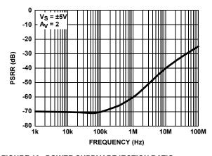
FIGURE 10. POWER SUPPLY REJECTION RATIO vs **FREQUENCY**
