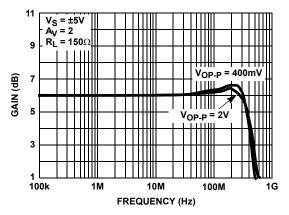
FIGURE 3. FREQUENCY RESPONSE vs OUTPUT VOLTAGE
