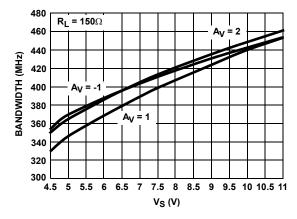
FIGURE 11. BANDWIDTH vs SUPPLY VOLTAGE
