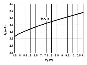
FIGURE 14. SUPPLY CURRENT vs SUPPLY VOLTAGE
