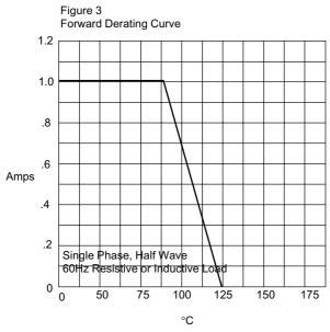
Average Forward Rectified Current - Amperes/ersus Ambient Temperature -  $^{\circ}$ C
