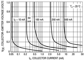
Figure 9. Collector Saturation Region
