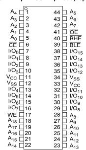
Figure 3. 48-pin TSOP I pinout (Top View) [1, 3]
