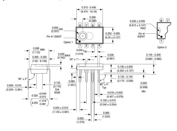
Molded Dual-In-Line Package (N) Package Number N08E
