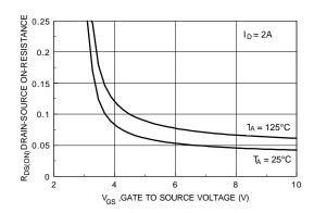
Figure 4. On-Resistance Variation with Gate-to-Source Voltage.
