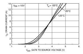
Figure 5. Transfer Characteristics.
