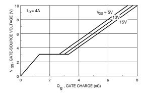
Figure 7. Gate Charge Characteristics.
