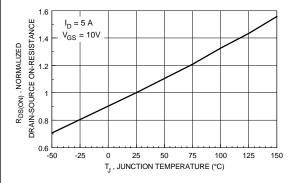
Figure 3. On-Resistance Variation with Temperature.
