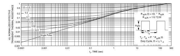
Figure 11. Transient Thermal Response Curve.
