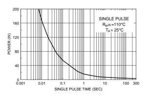
Figure 10. Single Pulse Maximum Power Dissipation.
