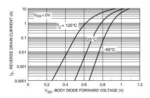
Figure 6. Body Diode Forward Voltage
