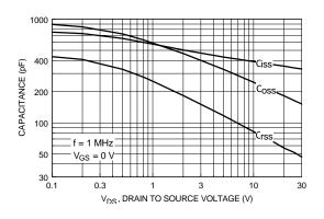
Figure 8. Capacitance Characteristics.
