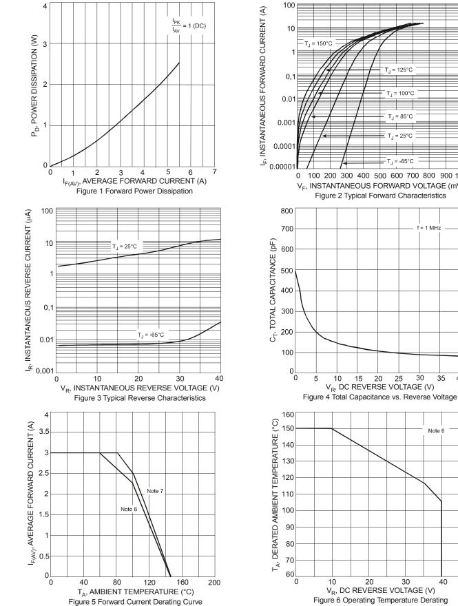
T<sub>1</sub> = 100°C T<sub>J</sub> = 85°C = 25°C ТJ T<sub>J</sub> = -65°C 100 200 300 400 500 600 700 800 900 1,000 V<sub>F</sub>, INSTANTANEOUS FORWARD VOLTAGE (mV) Figure 2 Typical Forward Characteristics : 1 MHz 25 30 35 20 40
