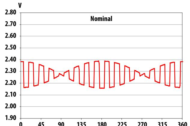
Figure 4. Output of D1 with code wheel eccentricity of 10  $\mu\text{m}$
