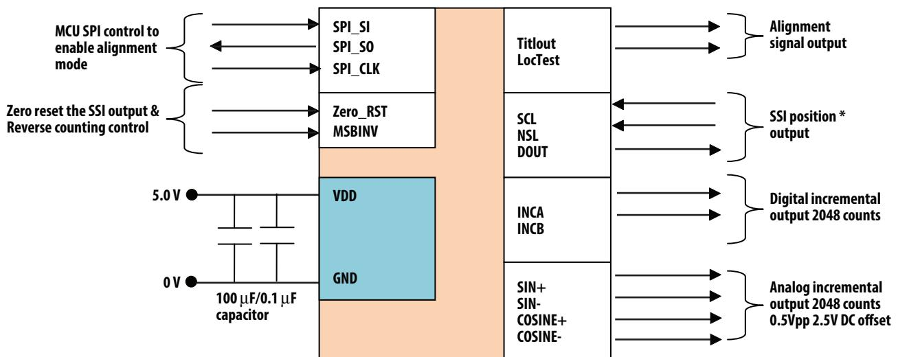
\* SCL, NSL and DOUT pins : reference to differential pins.
