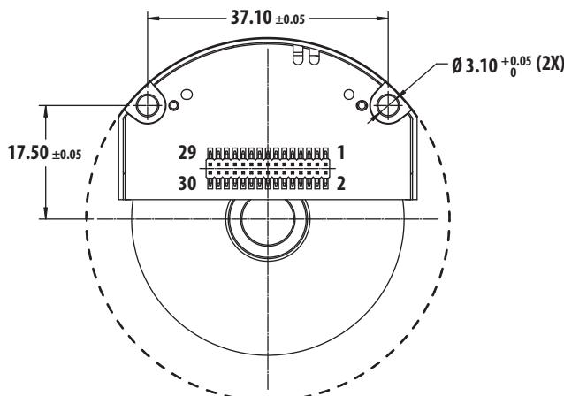
Figure 2. Alignment between read head and the codewheel.
