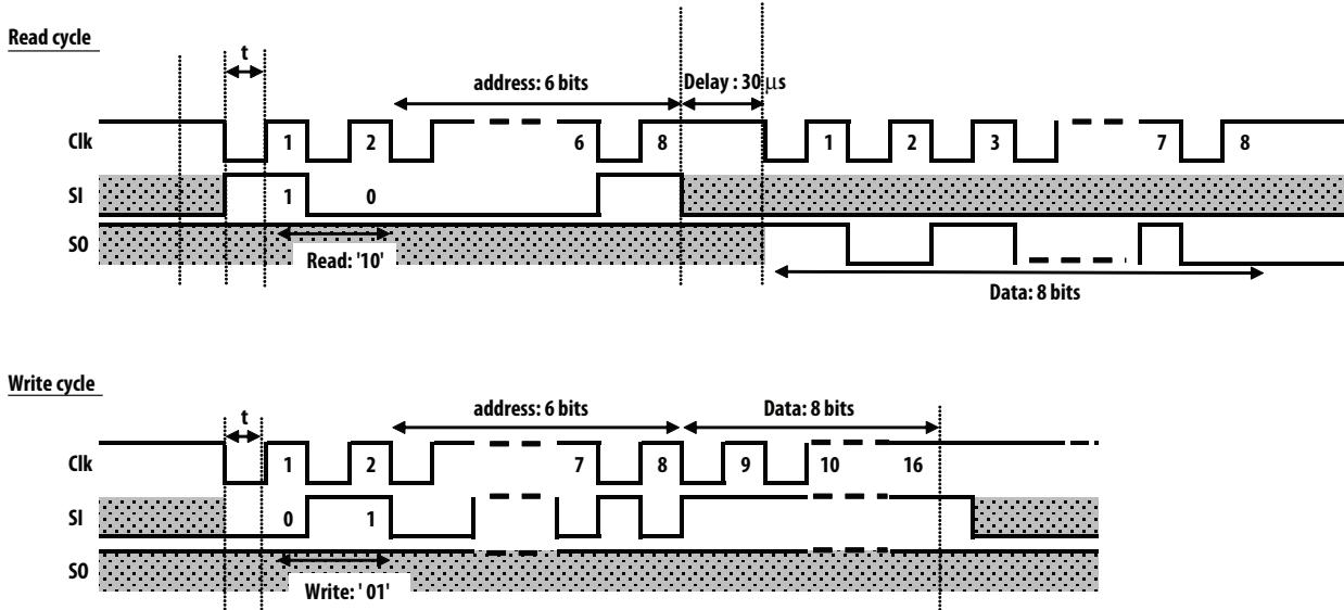
Figure 6. SPI timing diagram for read and write
