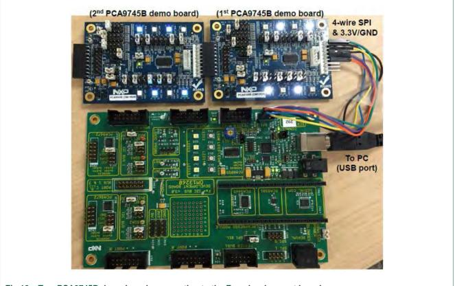
Fig 10. Two PCA9745B demo boards connecting to the Fm+ development board
