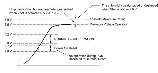
Figure 3. Understanding Integrated Circuit Voltage Limitations
