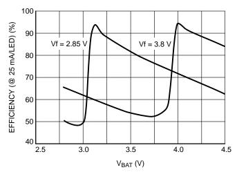
Figure 5. NCP5623C Typical Efficiency as a Function of the Vf
