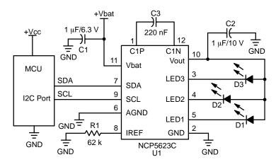
Figure 1. Typical Multiple White LED Driver
