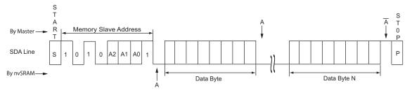
Figure 16. Current Location Single-Byte nvSRAM Read (Hs-mode)
