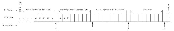
Figure 11. Multi-Byte Write into nvSRAM (except Hs-mode)
