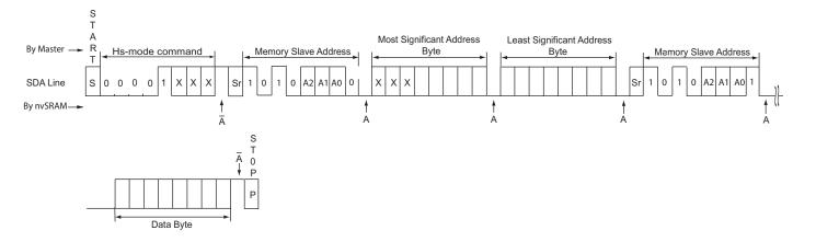
Figure 21. Random Address Multi-Byte Read (Hs-mode)
