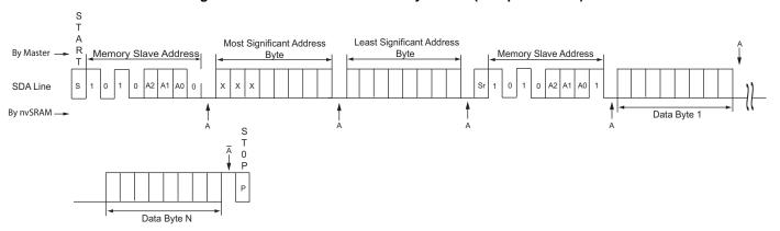
Figure 20. Random Address Single-Byte Read (Hs-mode)
