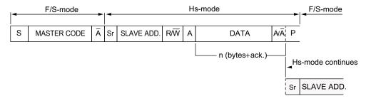
Single and multiple-byte reads and writes are supported. After the device enters Hs-mode, data transfer continues in Hs-mode until the stop condition is sent by the master device. The slave switches back to F/S-mode after a STOP condition (P). To continue data transfer in Hs-mode, the master sends Repeated START (Sr).
