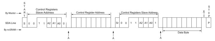
Figure 27. Random Control Registers Multi-Byte Read
