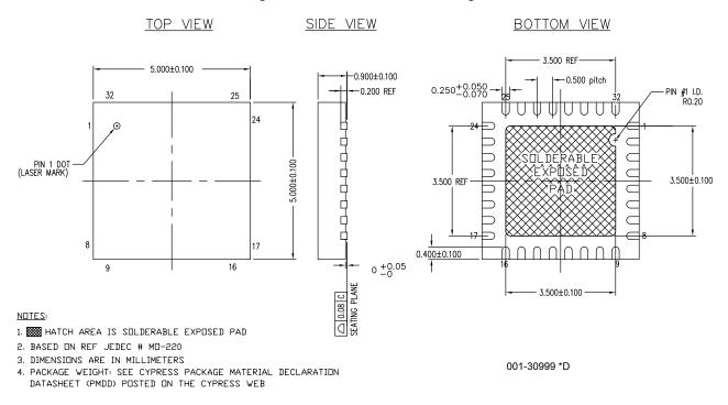
Figure 25. 32-Pin Sawn QFN Package
