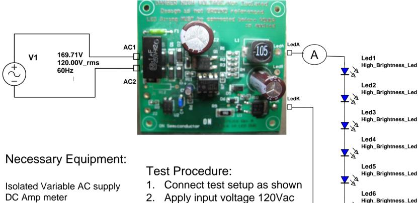
Output current can be reduced by removing some of the 5.1ohm parallel resistors (R1-R5)
