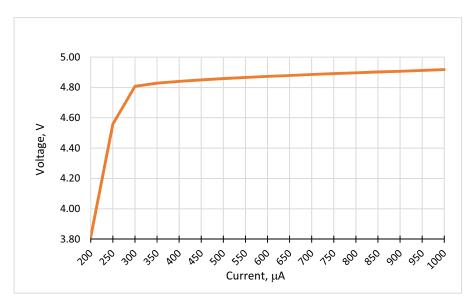
Figure 30. Typical I-V Curve for VREGA/B
