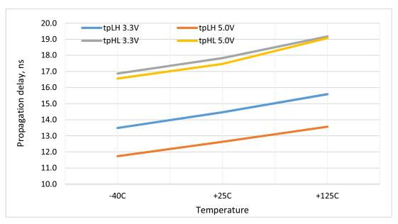
Figure 20. Propagation Delay vs. Temperature
