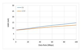
Figure 12. Si88241 Typical V<sub>DDA</sub> Supply Current vs. Data Rate (5 and 3.3 V Operation)
