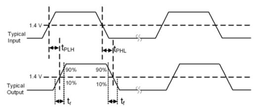
**Figure 1. Propagation Delay Timing for Digital Channels**
