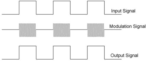
Figure 7. Modulation Scheme
