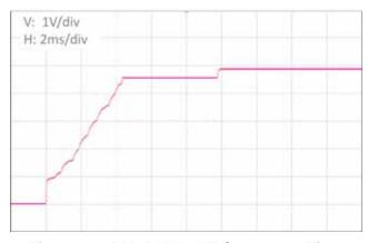
Figure 27. 5 V-5 V VOUT Startup vs.Time (50 mA Load Current)
