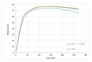
Figure 22. Efficiency vs. Load Current over Temperature (3.3 to 5.0 V)
