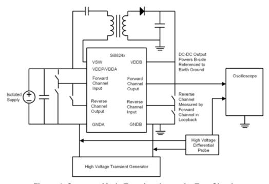
Figure 4. Common-Mode Transient Immunity Test Circuit
