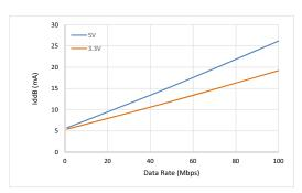
Figure 11. Si88240 Typical V<sub>DDB</sub> Supply Current vs. Data Rate (5 and 3.3 V Operation)
