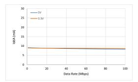
Figure 10. Si88240 Typical V<sub>DDA</sub> Supply Current vs. Data Rate (5 and 3.3 V Operation)
