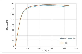
Figure 24. Efficiency vs. Load Current over Temperature (5.0 to 5.0 V)
