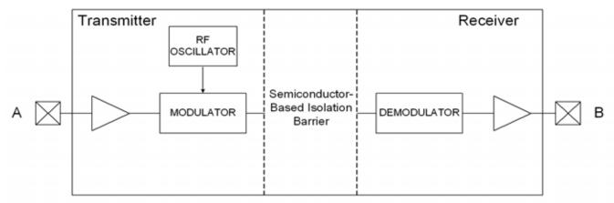
Figure 6. Simplified Si88xx Channel Diagram
