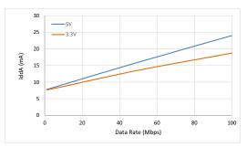
Figure 16. Si88243 Typical V<sub>DDA</sub> Supply Current vs. Data Rate (5 and 3.3 V Operation)
