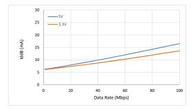
Figure 15. Si88242 Typical V<sub>DDB</sub> Supply Current vs. Data Rate (5 and 3.3 V Operation)
