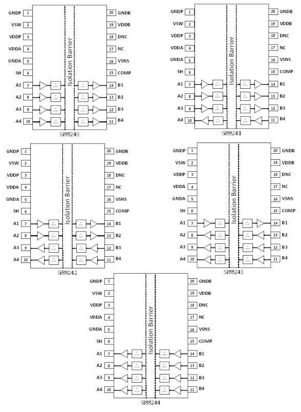
Figure 31. Si8824x Pin Configurations
