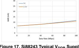
Figure 17. Si88243 Typical V<sub>DDB</sub> Supply Current vs. Data Rate (5 and 3.3 V Operation)
