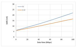
Figure 13. Si88241 Typical V<sub>DDB</sub> Supply Current vs. Data Rate (5 and 3.3 V Operation)
