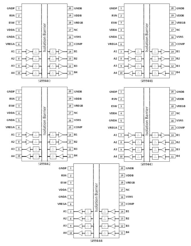
Figure 33. Si8844x Pinout Diagrams
