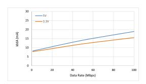
Figure 14. Si88242 Typical V<sub>DDA</sub> Supply Current vs. Data Rate (5 and 3.3 V Operation)
