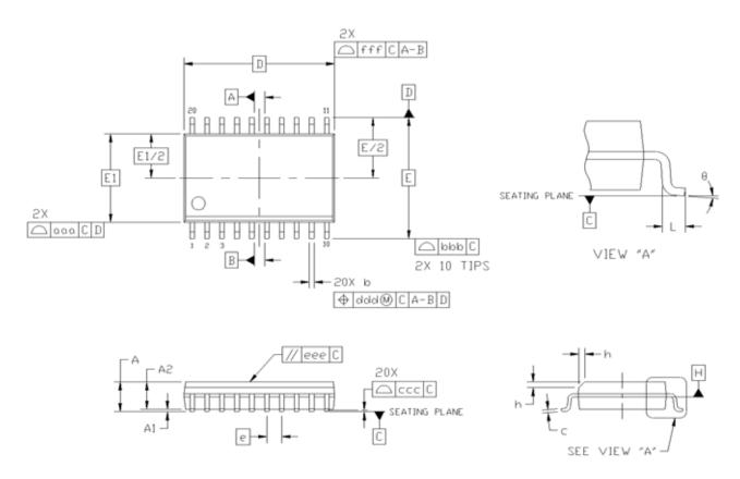
Figure 35. 20-Pin Wide Body SOIC
