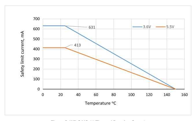
Figure 5. WB SOIC-20 Thermal Derating Curve\*
