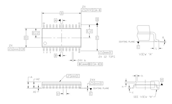
Figure 37. 24-Pin Wide Body SOIC
