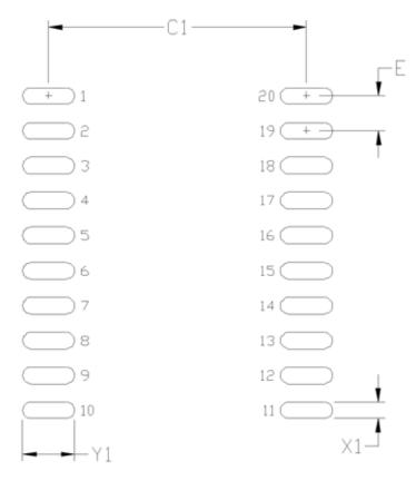
Figure 36. 20-Pin SOIC PCB Land Pattern
