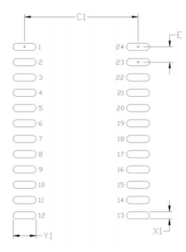
Figure 38. 24-Pin SOIC PCB Land Pattern
