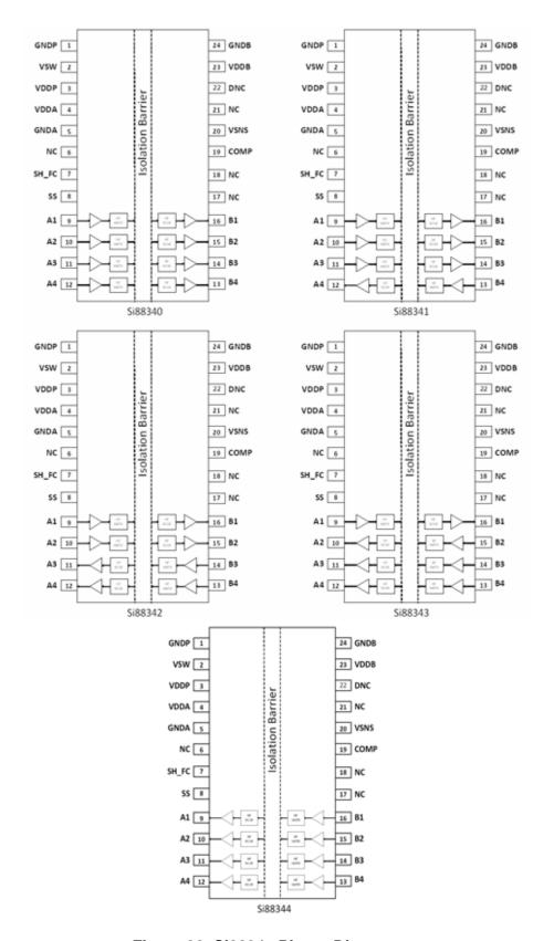
Figure 32. Si8834x Pinout Diagrams
