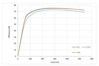
Figure 23. Efficiency vs. Load Current over Temperature (5.0 to 3.3 V)
