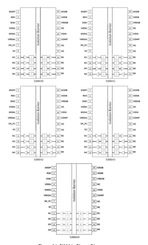
Figure 34. Si8864x Pinout Diagrams
