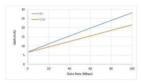
Figure 18. Si88244 Typical V<sub>DDA</sub> Supply Current vs. Data Rate (5 and 3.3 V Operation)
