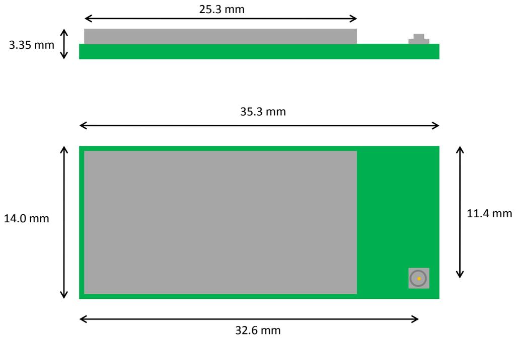
**Figure 6: Dimensions of WT41-E**
