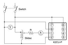
**Note:** Determine the value of R according to the specifications of the K2CU to be used. The dotted line indicates the connection at a supply voltage of 100 or 110 VAC.
