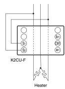
Note: The dotted lines which pass through the heater burnout detector indicate the line conductor passing through the round "window" of the window-type Current Transformer.
