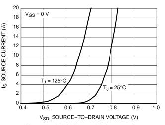
Figure 10. Diode Forward Voltage vs. Current
