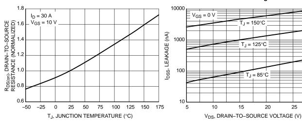
Figure 5. On–Resistance Variation with Temperature
