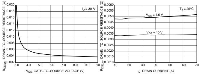
Figure 3. On-Resistance vs. V<sub>GS</sub>
