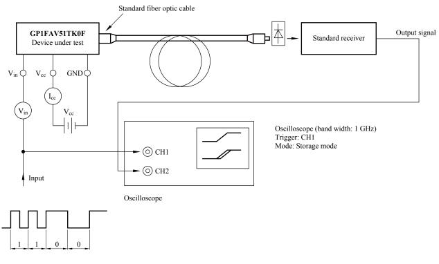
Input signal 6.6 Mb/s bi-phase PRBS signal
