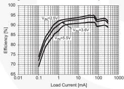
Figure 11. Efficiency vs. Load Current (V<sub>OUT</sub>=1.8V)
