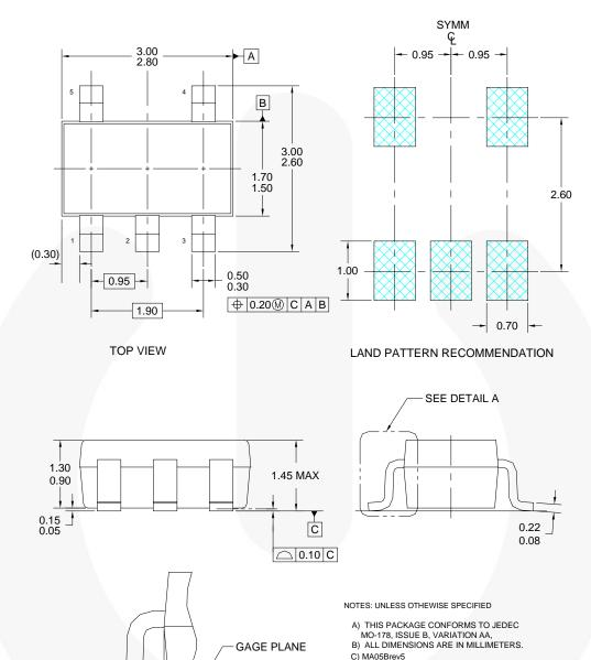
Figure 19. 5-Lead SOT-23 Package
