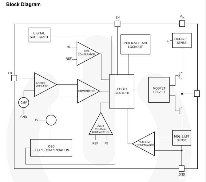
Figure 15. Block Diagram
