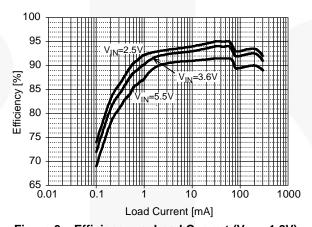
Figure 3. Efficiency vs. Load Current ( $V_{OUT}$ =1.8V)
