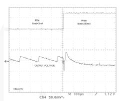
Figure 9. Load Transient Response
