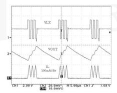
Figure 14. Power Save (PRM) Mode Operation
