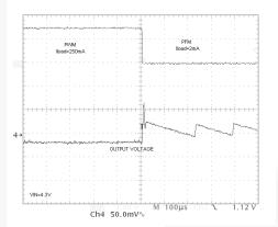
Figure 10. Load Transient Response
