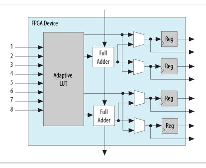
You can configure up to 50% of the ALMs in the Arria V devices as distributed memory using MLABs.
