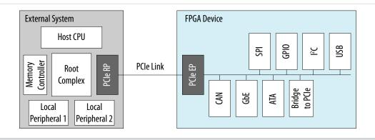
The Arria V PCIe hard IP operates independently from the core logic. This independent operation allows the PCIe link to wake up and complete link training in less than 100 ms while the Arria V device completes loading the programming file for the rest of the device.
