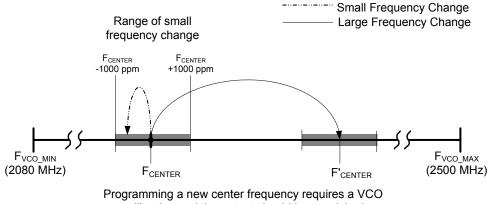
calibration and the output should be squelched
