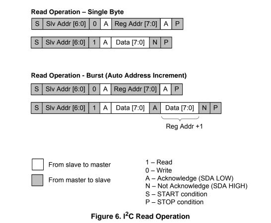
The timing specifications and timing diagram for the  $I^2C$  bus is compatible with the  $I^2C$ -Bus standard. SDA timeout is supported for compatibility with SMBus interfaces.
