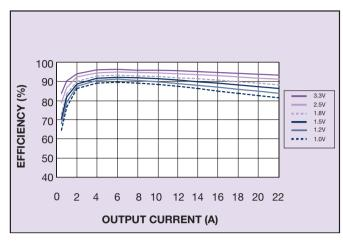
Figure 2 - Efficiency vs Load Current Vin = 5 V (See Note B)
