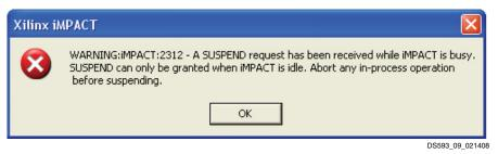
Figure 9: Suspend Warning When iMPACT (10.1 or later) is Busy
