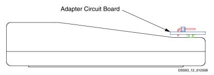
Figure 12: Flying Wire Adapter (Side) without Wires
