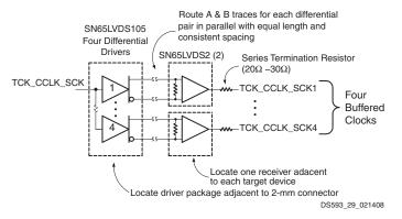
Figure 29: Differential Clock Buffer Example
