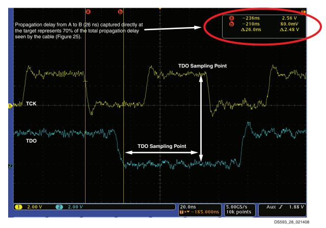
Figure 28: TDO Sampling Example at 12 MHz (Analog Signals on Target System)
