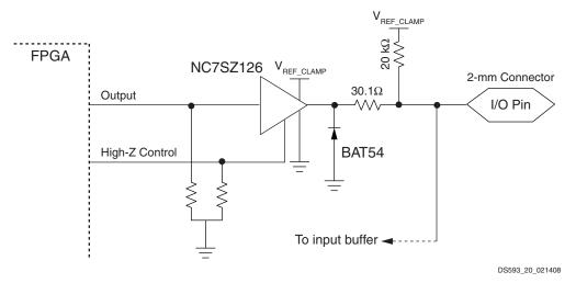
Figure 20: Target Interface Driver Topology
