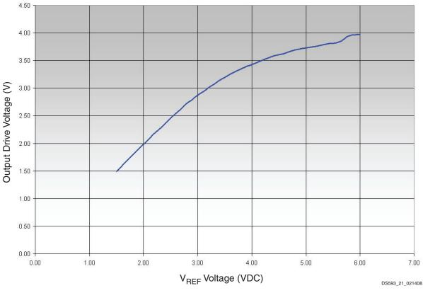
Figure 21: Output Drive Voltage vs. V<sub>REF</sub>
