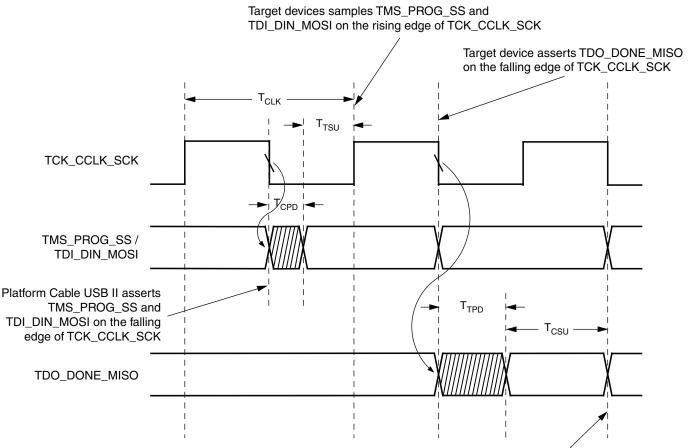
Platform Cable USB II samples TDO\_DONE\_MISO on the falling edge of TCK\_CCLK\_SCK
