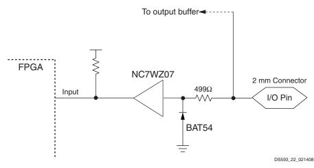
Figure 22: Target Interface Receiver Topology
