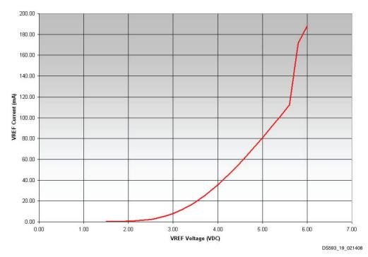
Figure 19: V<sub>REF</sub> Current vs. V<sub>REF</sub> Voltage
