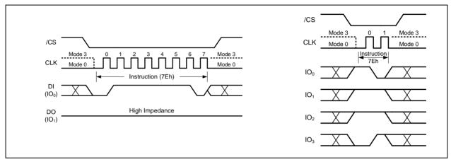
Figure 54. Global Block Lock Instruction for SPI Mode (left) or QPI Mode (right)
