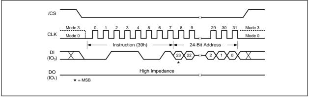
Figure 52a. Individual Block Unlock Instruction (SPI Mode)
