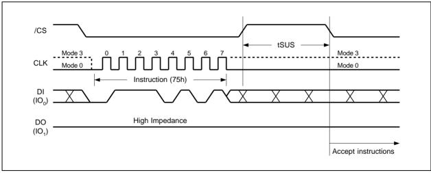
Figure 35a. Erase/Program Suspend Instruction (SPI Mode)
