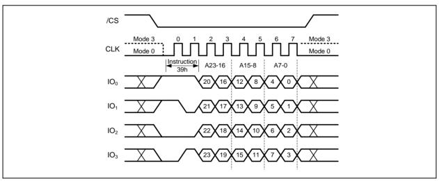
Figure 52b. Individual Block Unlock Instruction (QPI Mode)
