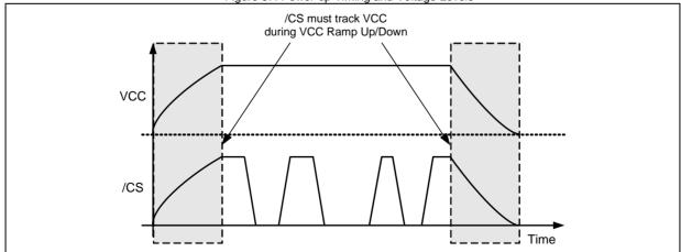
Figure 57a. Power-up, Power-Down Requirement
