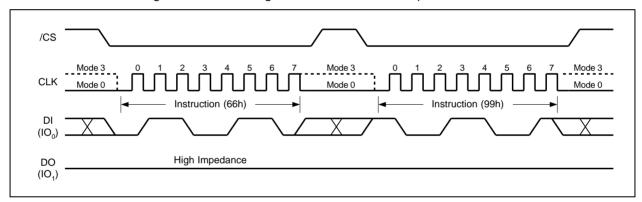
Figure 56a. Enable Reset and Reset Instruction Sequence (SPI Mode)
