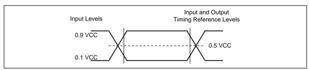
Figure 58. AC Measurement I/O Waveform
