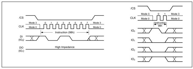
Figure 55. Global Block Unlock Instruction for SPI Mode (left) or QPI Mode (right)
