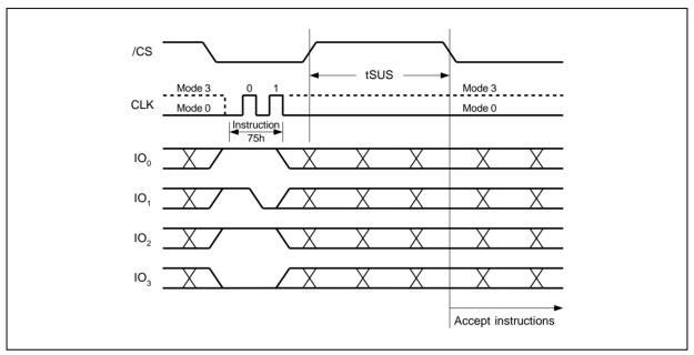
Figure 35b. Erase/Program Suspend Instruction (QPI Mode)
