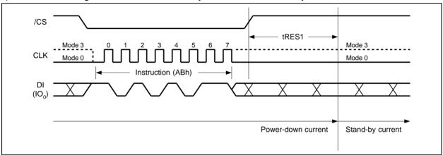
Figure 38a. Release Power-down Instruction (SPI Mode)
