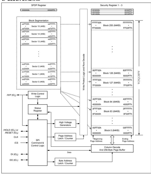
Figure 2. W25Q128FW Serial Flash Memory Block Diagram
