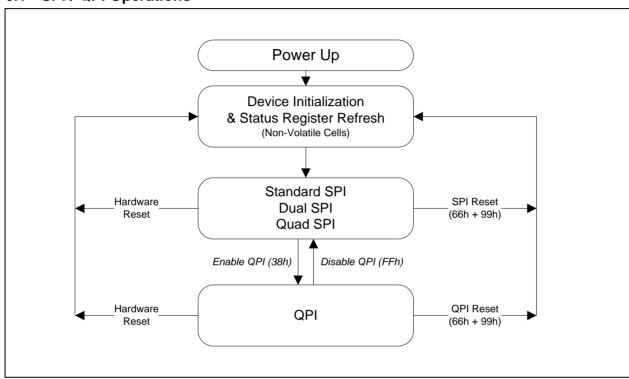
Figure 3. W25Q128FW Serial Flash Memory Operation Diagram
