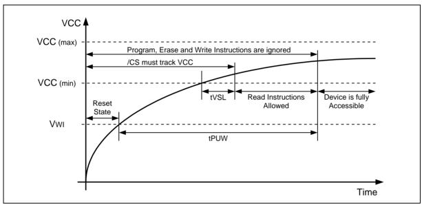
Figure 57. Power-up Timing and Voltage Levels
