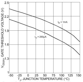
Figure 8 Gate Threshold Variation vs. Ambient Temperature
