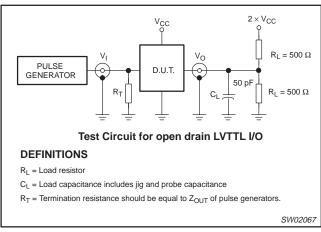
Figure 6. Load circuitry for open drain LVTTL I/O
