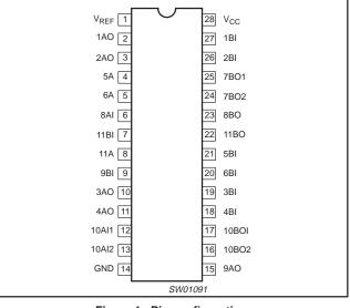
Figure 1. Pin configuration
