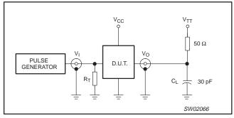
Figure 7. Load circuit for B outputs
