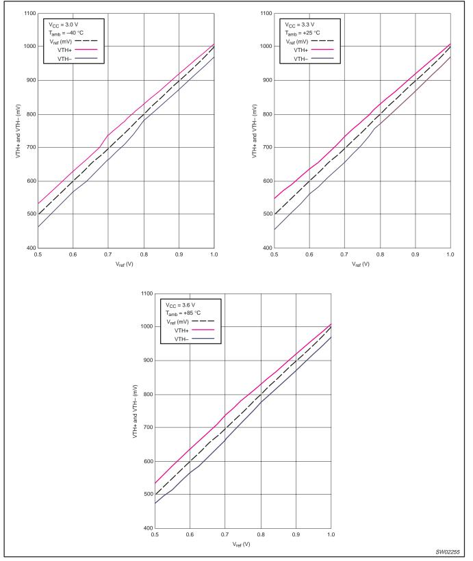
Figure 4. GTL  $V_{TH+}$  and  $V_{TH-}$  versus  $V_{REF}$
