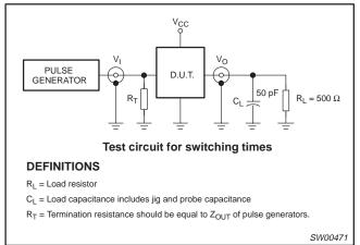
Figure 5. Load circuitry for A outputs
