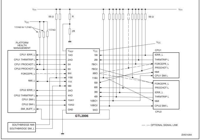
Figure 3. Application diagram
