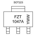
FZT 1047A = Product Type Marking Code YWW = Date Code Marking Y or  $\overline{Y}$  = Last Digit of Year (ex: 5= 2015) WW or  $\overline{W}W$  = Week Code (01~53)
