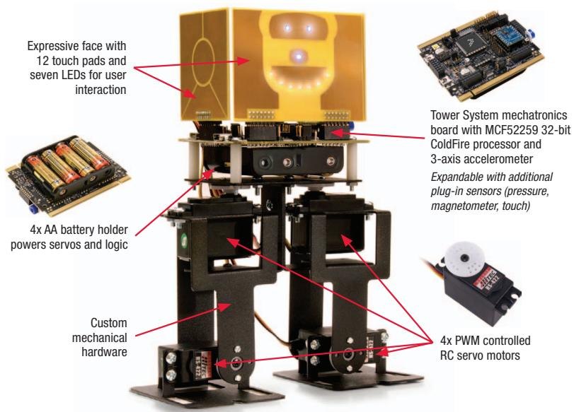
Tower System mechatronics board with MCF52259 32-bit ColdFire processor and 3-axis accelerometer
