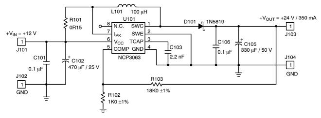
Figure 19. Typical Boost Application Schematic
