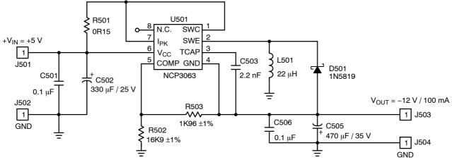
Figure 22. Typical Voltage Inverting Application Schematic
