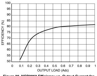
Figure 30. NCP3063 Efficiency vs. Output Current for External Low  $V_{CE(sat)}$  at  $V_{in}$  = +5 V, f = 160 kHz, T<sub>A</sub> = 25°C
