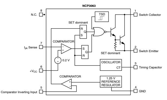
Figure 4. Block Diagram
