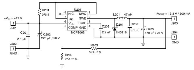
Figure 16. Typical Buck Application Schematic
