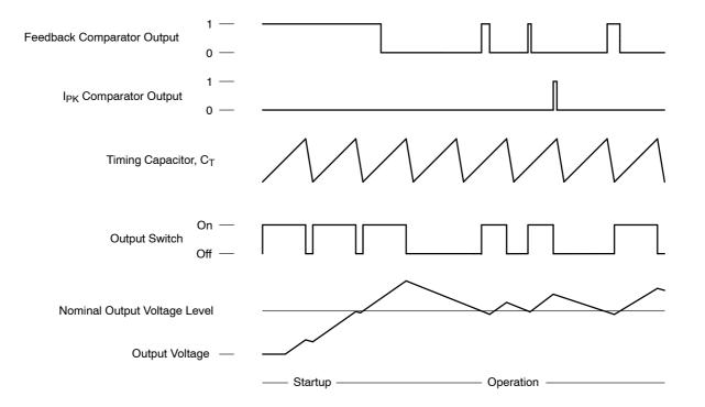
Figure 14. Typical Operating Waveforms
