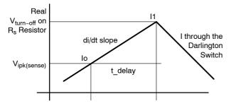
The  $V_{IPK(Sense)}$  Current Limit Sense Voltage threshold is specified at static conditions. In dynamic operation the sensed current turn-off value depends on comparator response time and di/dt current slope.
