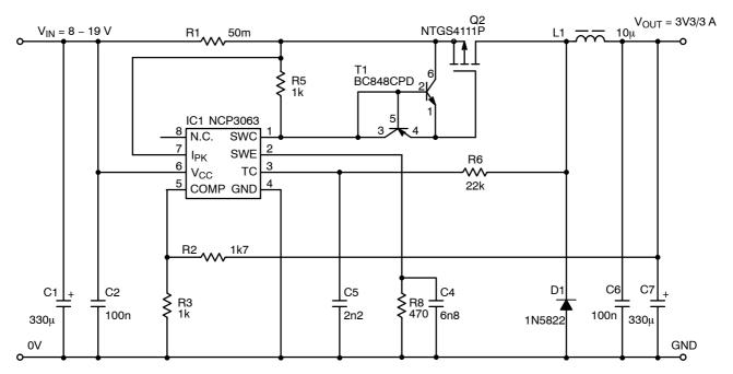
Figure 27. Typical Buck Application Schematic with External PMOS Transistor
