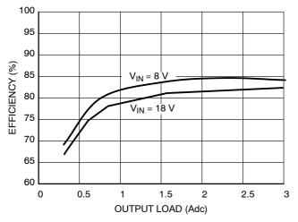
Figure 28. NCP3063 Efficiency vs. Output Current for Buck External PMOS at V<sub>out</sub> = 3.3 V, f = 220 kHz,  $T_A = 25^{\circ}C$
