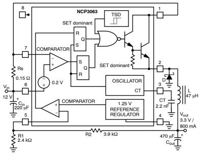
Figure 1. Typical Buck Application Circuit
