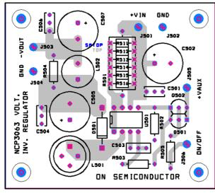
Figure 23. Voltage Inverting Demoboard Layout
