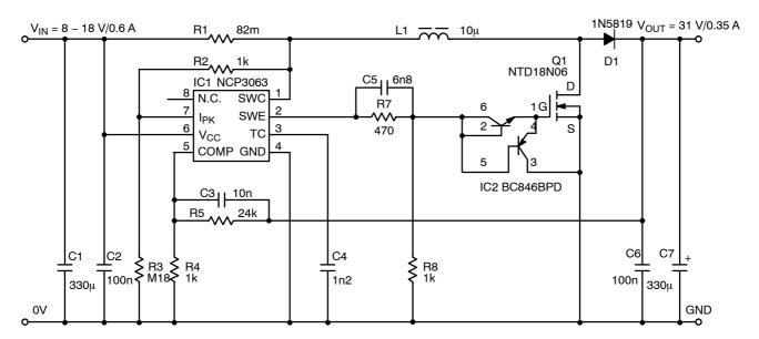
Figure 25. Typical Boost Application Schematic with External NMOS Transistor
