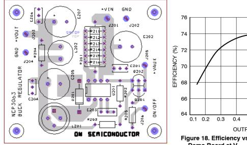
Figure 17. Buck Demoboard Layout
