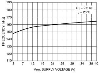
Figure 6. Oscillator Frequency vs. Supply Voltage
