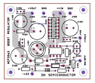
Figure 20. Boost Demoboard Layout
