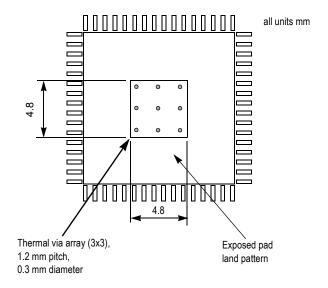
Figure 6. Recommended Thermal Land Pattern
