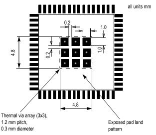
Figure 7. Recommended Solder Mask Openings
