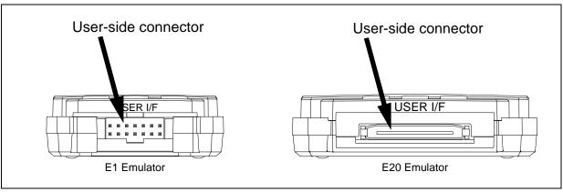
Figure 2.2 User-Side Connector on the E1 and E20
