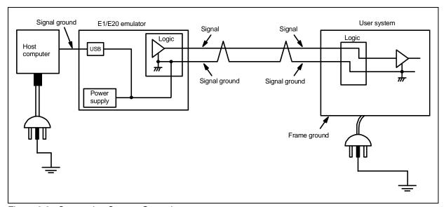
Figure 2.6 Connecting System Ground
