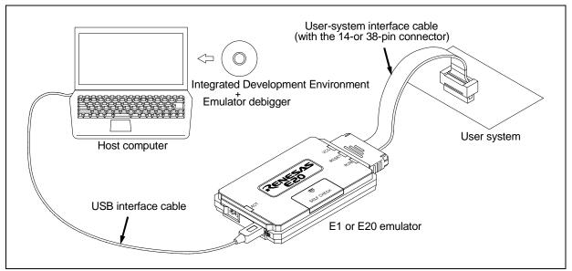
Figure 1.1 System configuration with an Emulator
