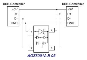
Figure 1. USB 2.0 High Speed Port
