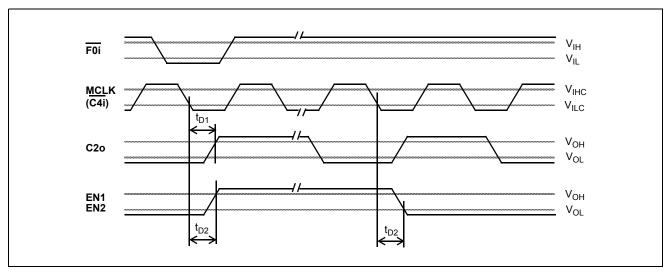
Figure 15 - ST-BUS Timing for External Signal Generation
