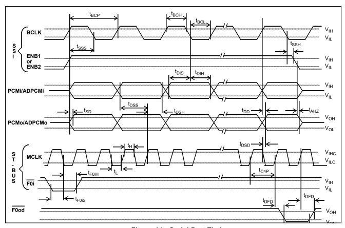
Figure 14 - Serial Port Timing
