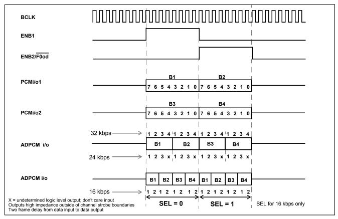
Figure 4 - SSI 8-Bit Companded PCM Relative Timing
