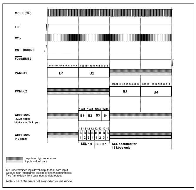
Figure 8 - ST-BUS 16-Bit Linear PCM Relative Timing
