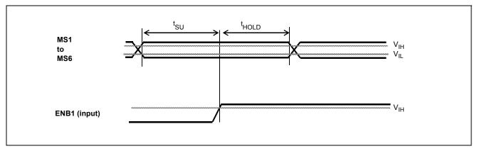
Figure 16 - SSI Mode Select Set-up and Hold Timing
