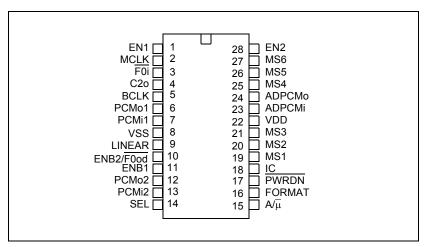
Figure 2 - Pin Connections
