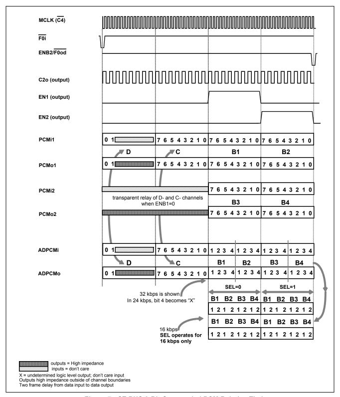
Figure 7 - ST-BUS 8-Bit Companded PCM Relative Timing
