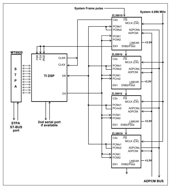
Figure 13 - ST-BUS to DSP Platform
