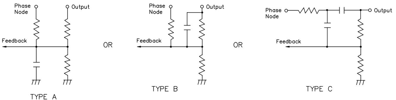
The phase injection improves stability and can provide droop response.
